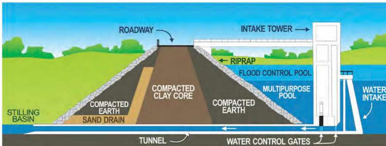
FIGURE 2.1. EMBANKMENT DAM (U.S. ARMY CORPS OF ENGINEERS).
